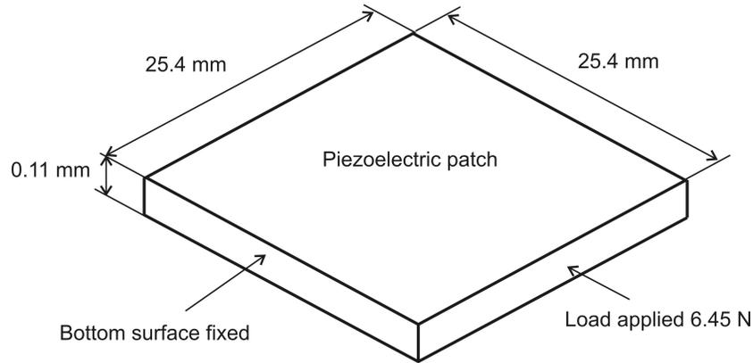
Fig. 1. Piezo film subjected to load.
